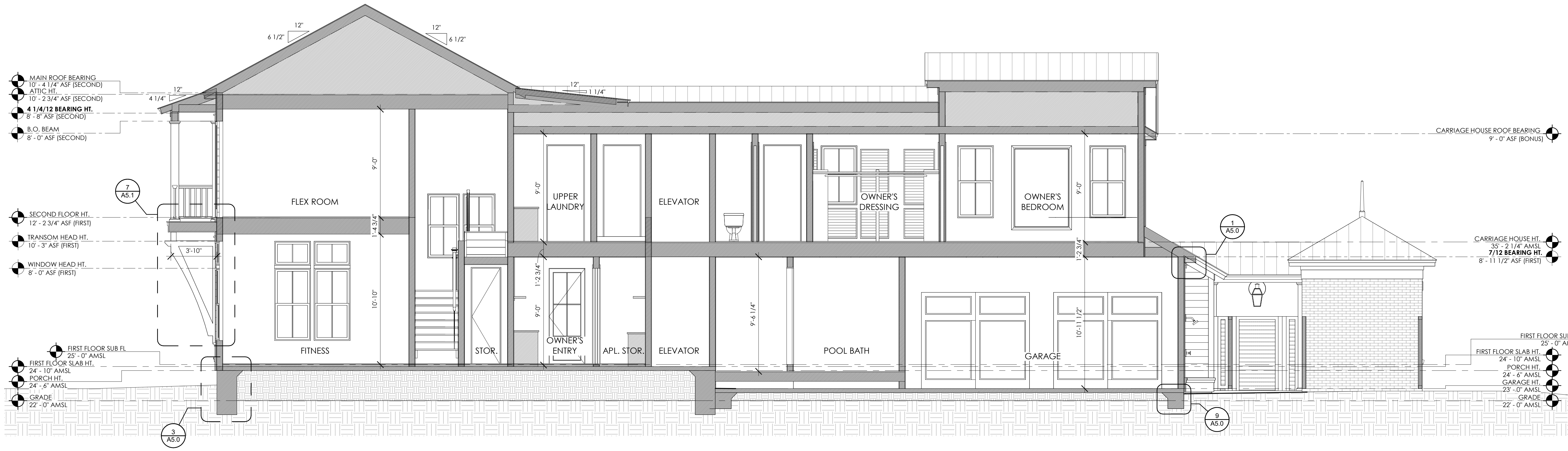
1 SECTION AT CARRIAGE HOUSE A4.1 1/4\" = 1'-0"
