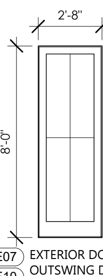
E07 EXTERIOR DOOR SYSTEM (MATERIAL T.B.D.) OUTSWINGING DOOR W/ TRANSOM 2'-8" x 8'-0" (R.O. ±) SDL MUNTINS W/ SPACE BAR (PATTERN AS SHOWN) MANUFACTURER T.B.D. BY G.C. / OWNER DP RATING 50 OR APPROVED EQUIVALENT
