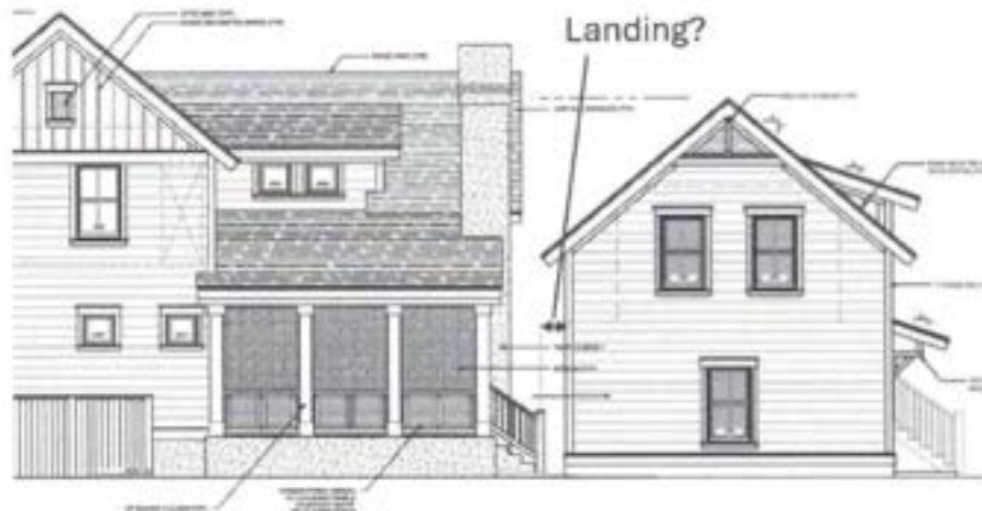
Fig 3. – Location of a Landing (possible code infraction)
