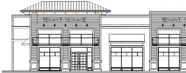
May River Crossing Existing Building – 45% of façade has partial metal roof features - a flat roof is behind the angled metal roof sections
