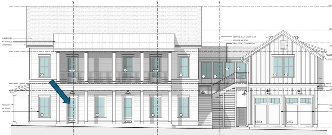
Fig 1. Door Replacement on West Elevation
