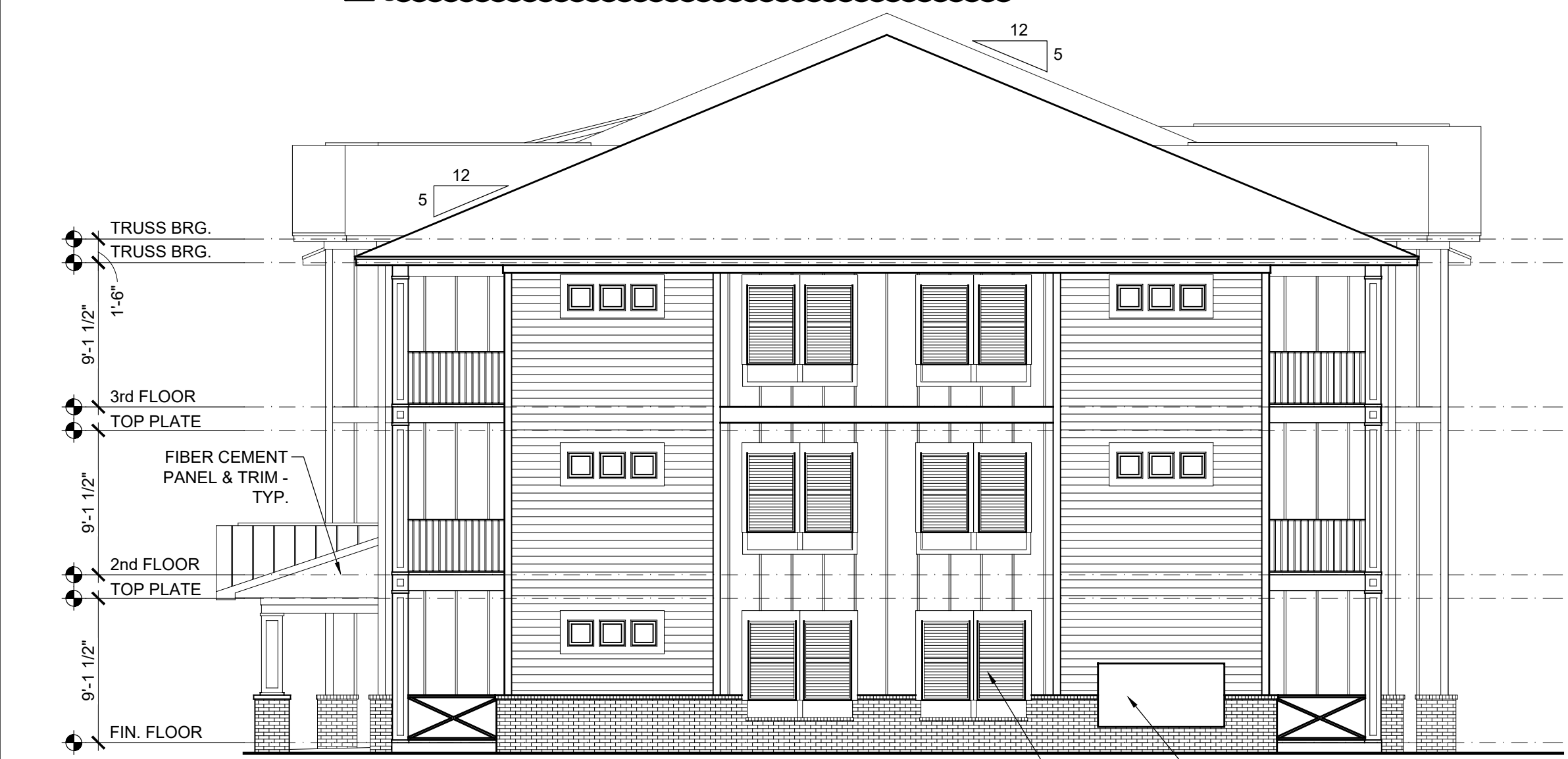
3 BUILDING TYPE "C" RIGHT SIDE ELEVATION 1/8" = 1'-0"
