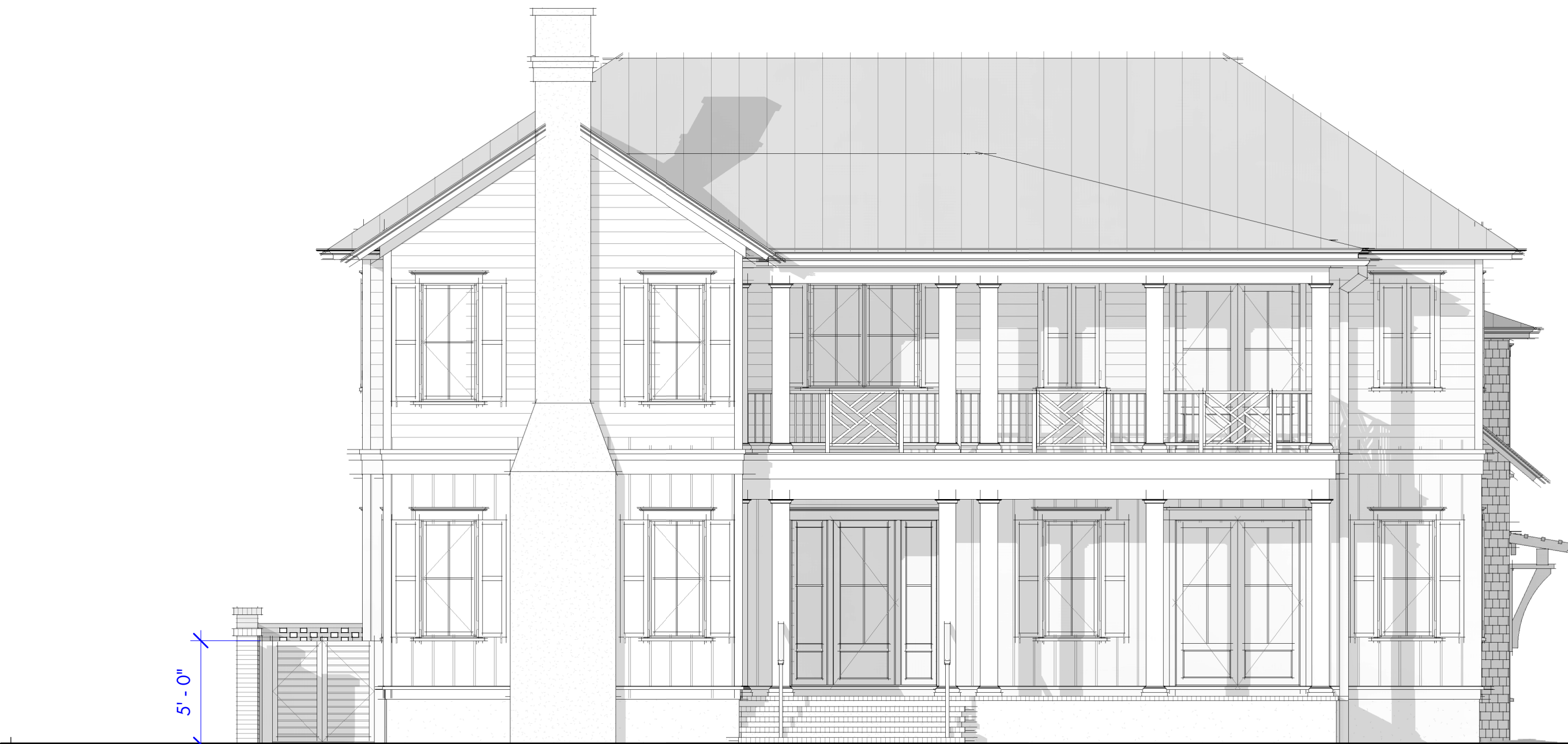
1 FRONT ELEVATION A3.2 3/16" = 1'-0"
