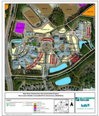
Figure 52. McCracken Middle School/Bluffton Elementary School Proposed Stormwater BMP Retrofits
