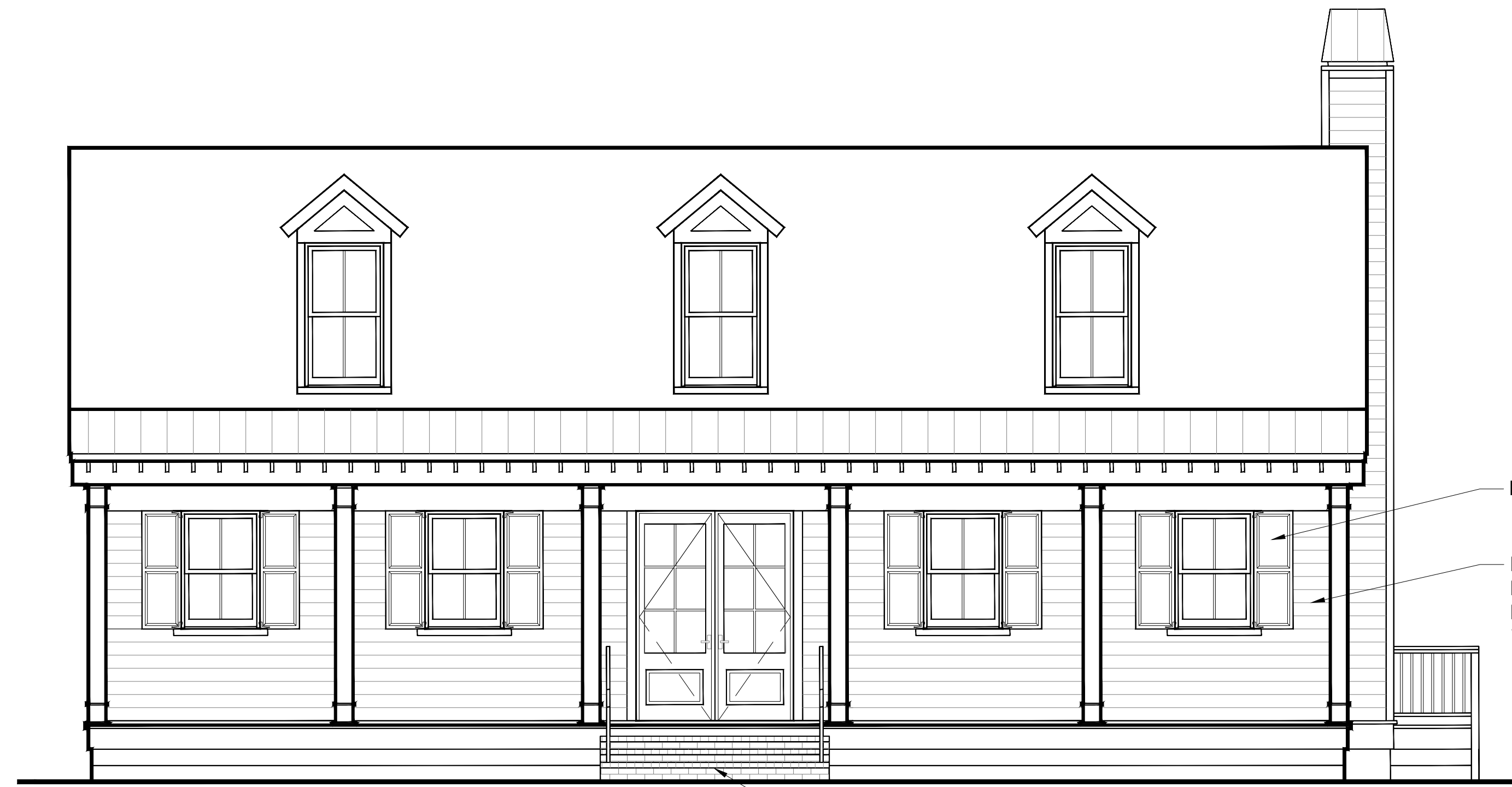
A A4 PROPOSED FRONT ELEVATION SCALE: 1/4"=1'-0"
