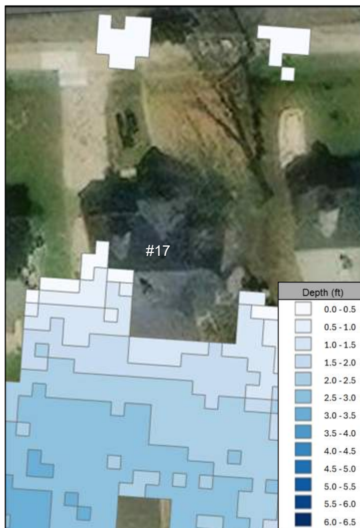
Figure 2.17.2.1 Property #17: 100-year flood depth above grade
