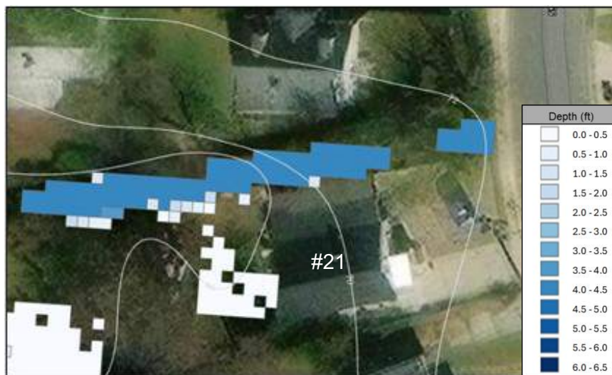
Figure 2.21.2.1 Property #21: 100-year flood depth above grade
