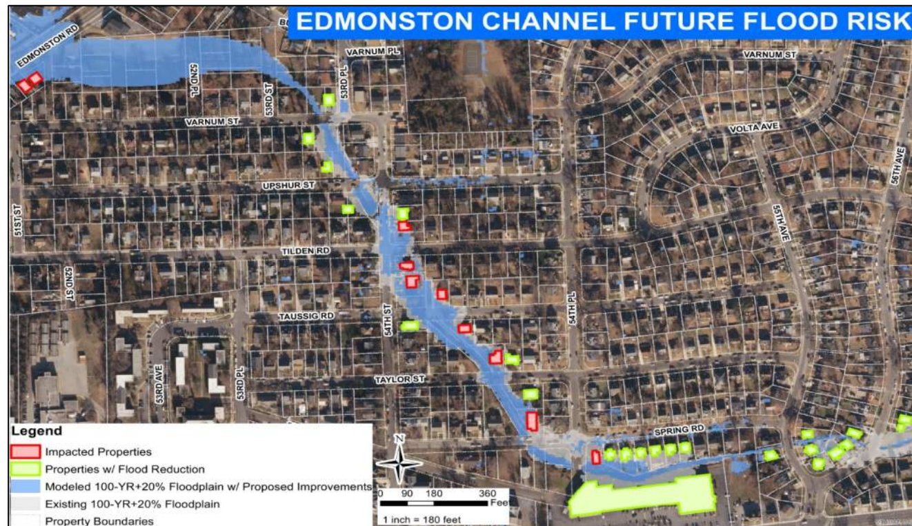
Figure 2-1 Edmonston Channel 100-yr + 20% Flood Risk
