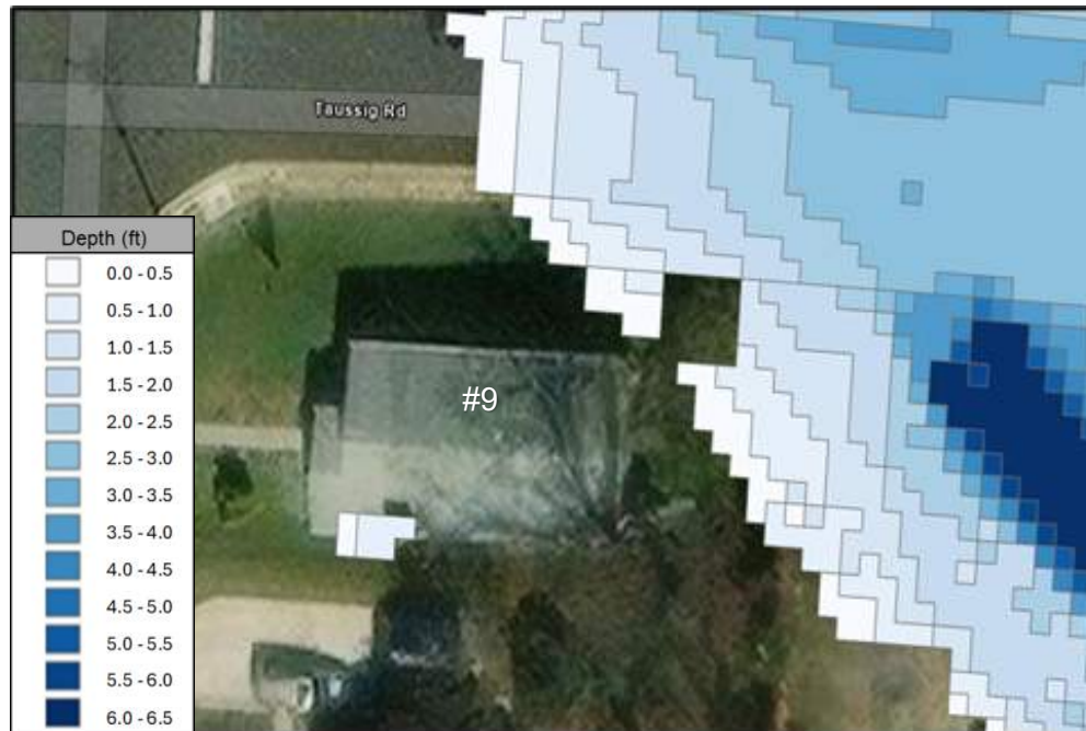
Figure 2.9.2.1 Property #9: 100-year flood depth above grade
