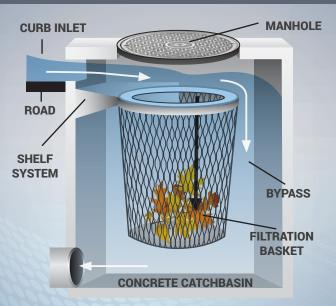
Curb inlet baskets (CIBs) help capture debris — such as dirt, leaves and trash — before it enters our lakes. If not captured, the debris can transport harmful chemicals into lakes and contribute to algal blooms caused by nutrient overloading.
