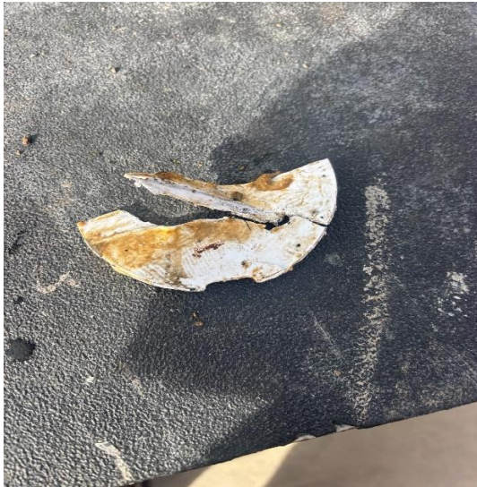
Oliver lift station pump failure due to plastic cap blocking the pump.
