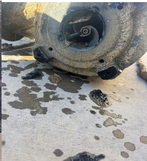
Oliver lift station pump failure due to plastic cap blocking the pump.
