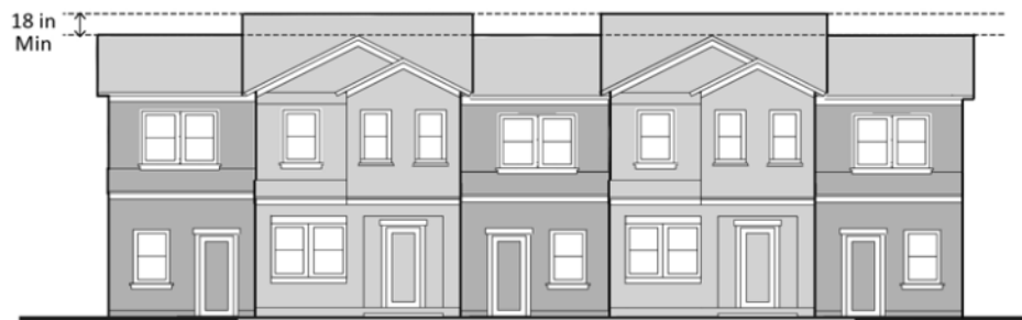
The roof line for each elevation shall be offset at least 18 inches for each one to three units exposed on that elevation.
