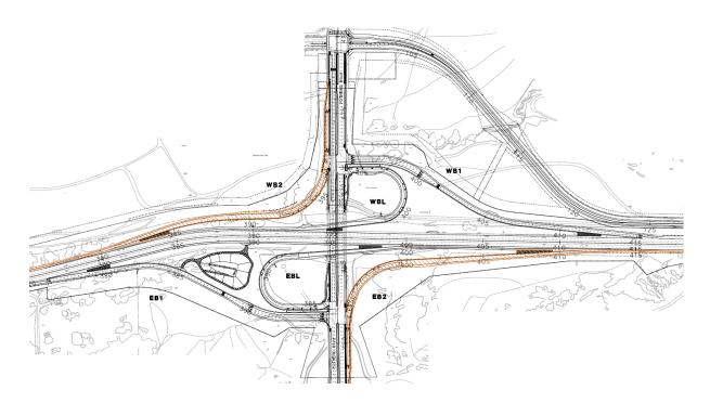
The ramps which are delineated in orange would be either deferred until warranted by future traffic, or eliminated altogether. In order to determine whether or not the ramps can be eliminated, a revised traffic analysis must be performed. Should the results of the analysis show that the failure year of the ramps would not occur within 15 years, Caltrans would be able to support removal based upon feedback provided in several focus meetings.
