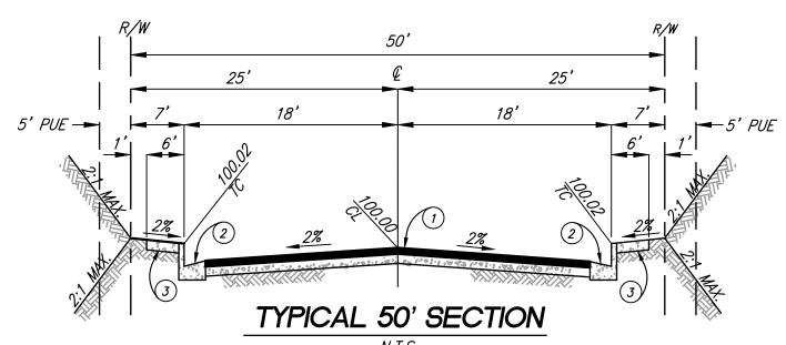
COUPLES COURT, FORD STREET, JOSH DRIVE AND SUGGS COURT MODIFIED RIVERSIDE COUNTY STD. 106, SECTION A T.I. = 5.5, 0.33' A.C. W/SEAL COAT OVER 0.50' A.B. CRUSHED PRELIM. "R" VALUE = 30
