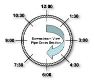
Figure 2-1 Clock Positions on Pipe Looking Downstream
