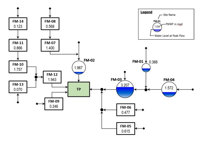
Figure 3-13. Peak Measured Flow (Flow Schematic)
