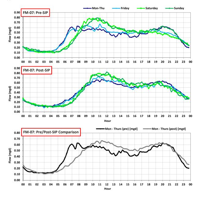
Figure 3-10. FM-07: pre-SIP and post-SIP Average Dry Weather Flow Curves with Comparison
