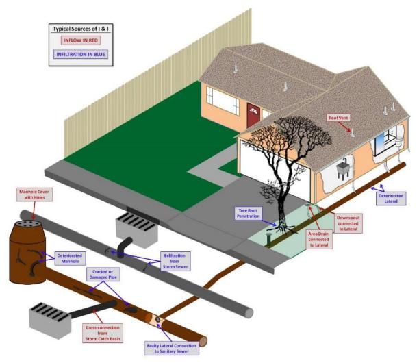
Figure 2-4 illustrates the possible sources and components of I/I.
