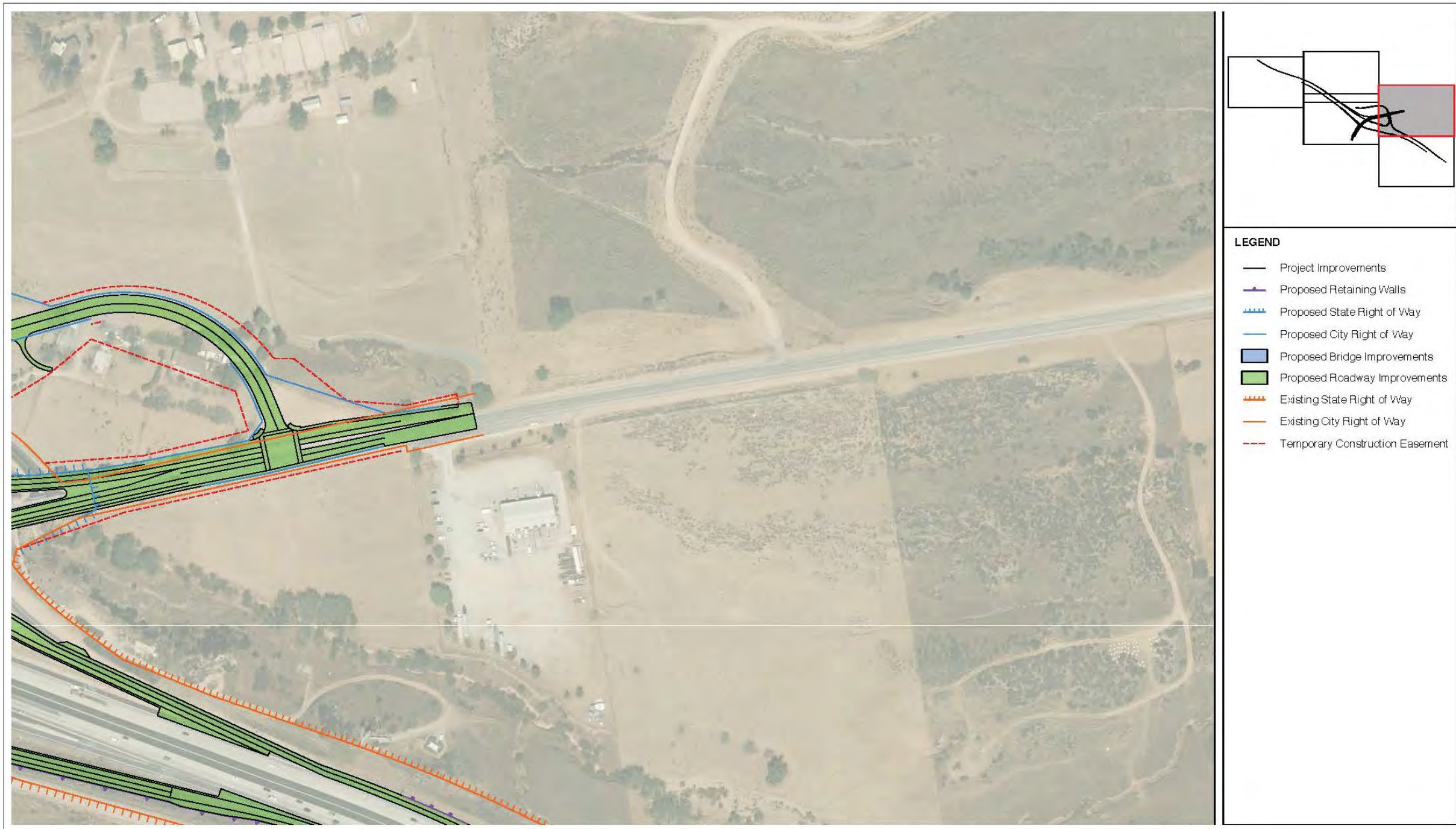
Figure 1-5d: Build Alternative 4 (Partial Cloverleaf)
