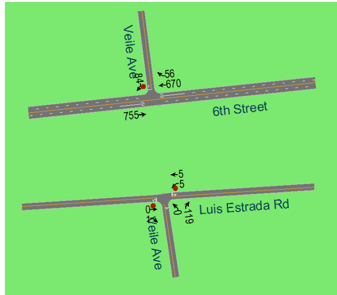
Figure 16 – PM Peak Hour Volumes with the Proposed Veile Ave Roadway Segment Closure Between 6 th St and Luis Estrada Rd
