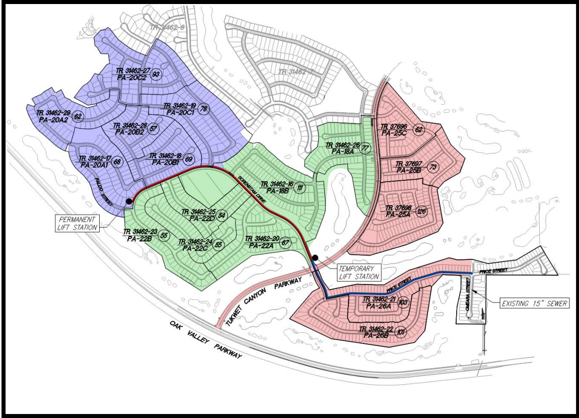
Figure 2 - Lift Station Location
