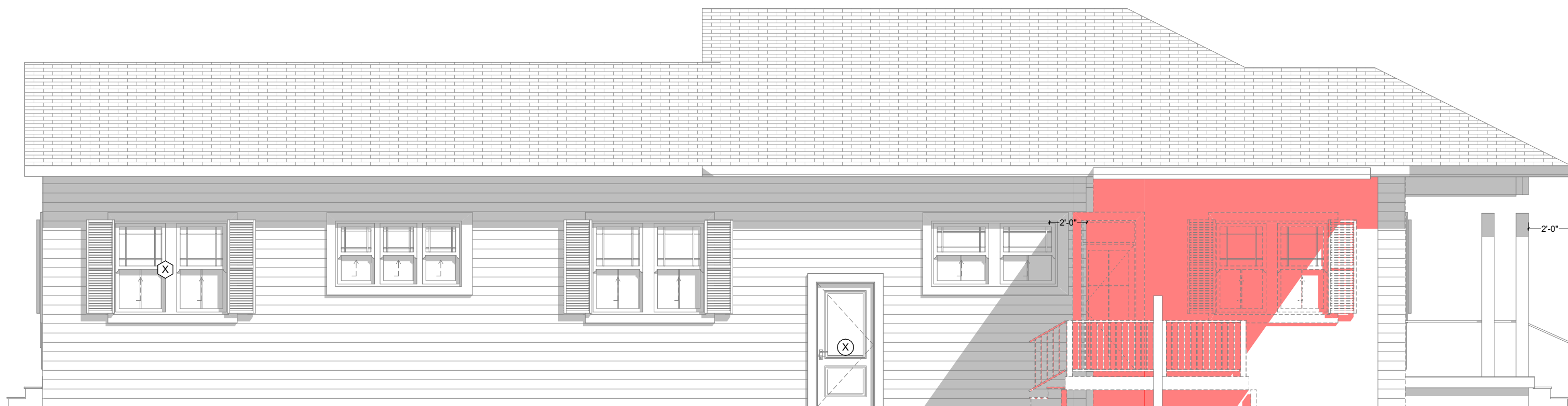
2 West Elevation Demolition Plan SCALE: 3/16" = 1'-0"
