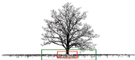
Figure 2. Tree roots most important for survival are the structural root plate (red area) and the critical root area (green area).
