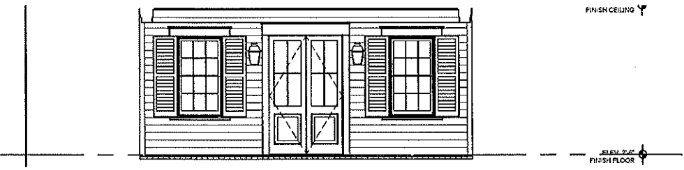
02.1 EXTERIOR ELEVATION - SCREEN PORCH SCALE 1/4" = 1'-0"
