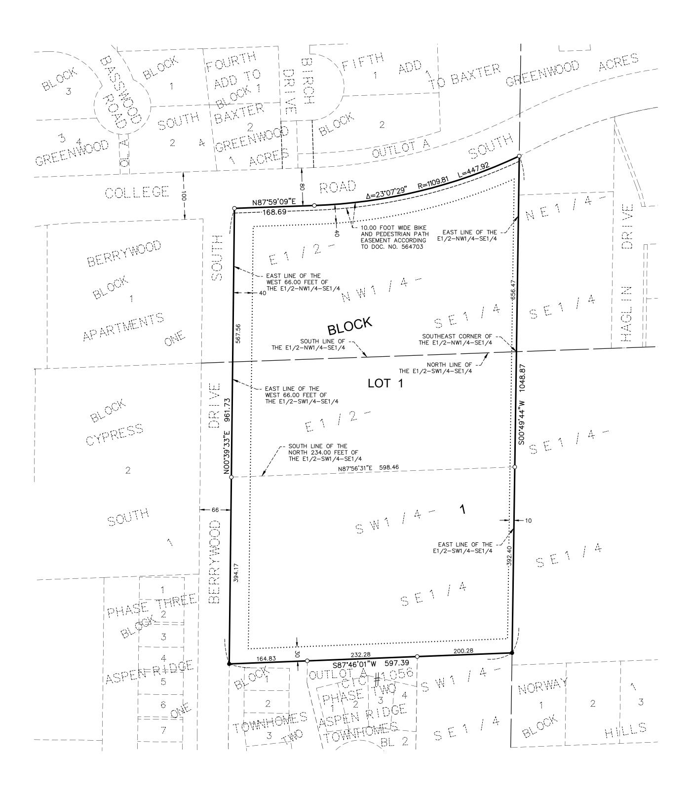
DRAINAGE AND UTILITY EASEMENTS ARE AS SHOWN BELOW INTERIOR SIDE J∣∟ \_\_ \_**!**-ROAD LINE ' BEING 5 FEET IN WIDTH AND ADJOINING ALL INTERIOR SIDE LOT LINES AND 10 FEET IN WIDTH AND ADJOINING ALL ROAD LINES
