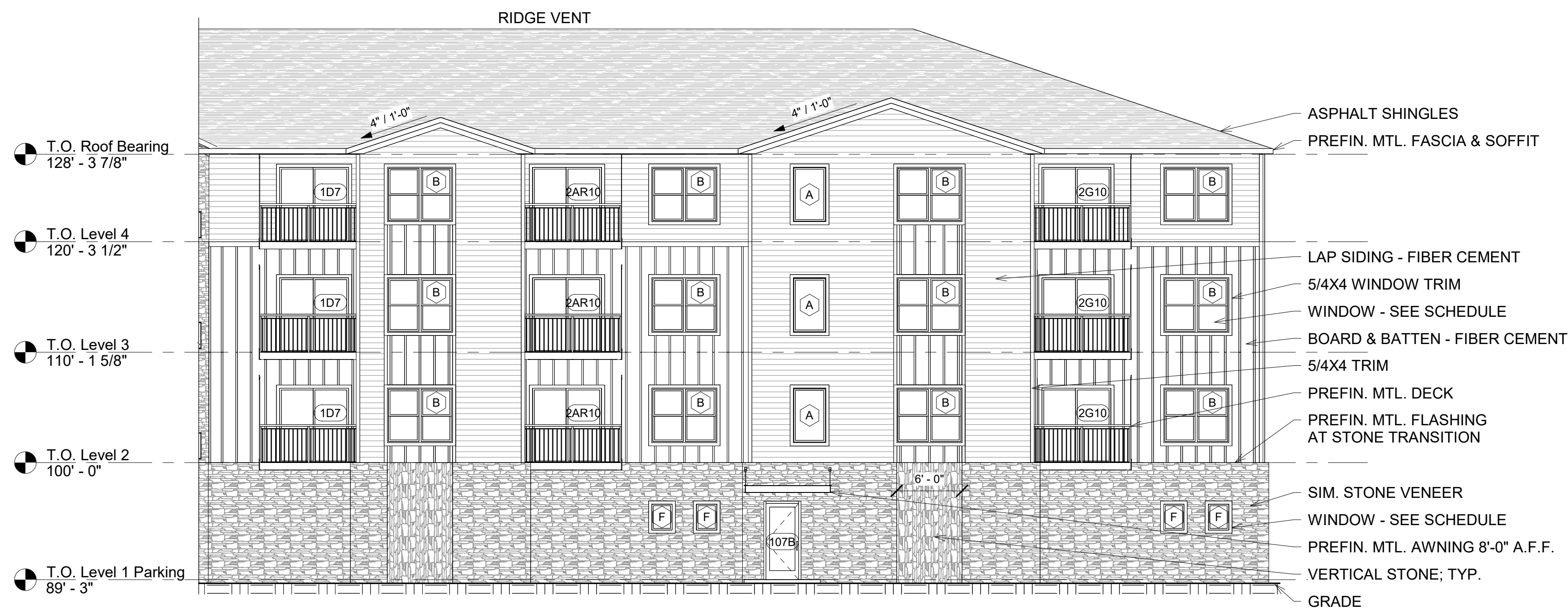
2 Enlarged Building Elevation - West 2 1/8" = 1'-0"
