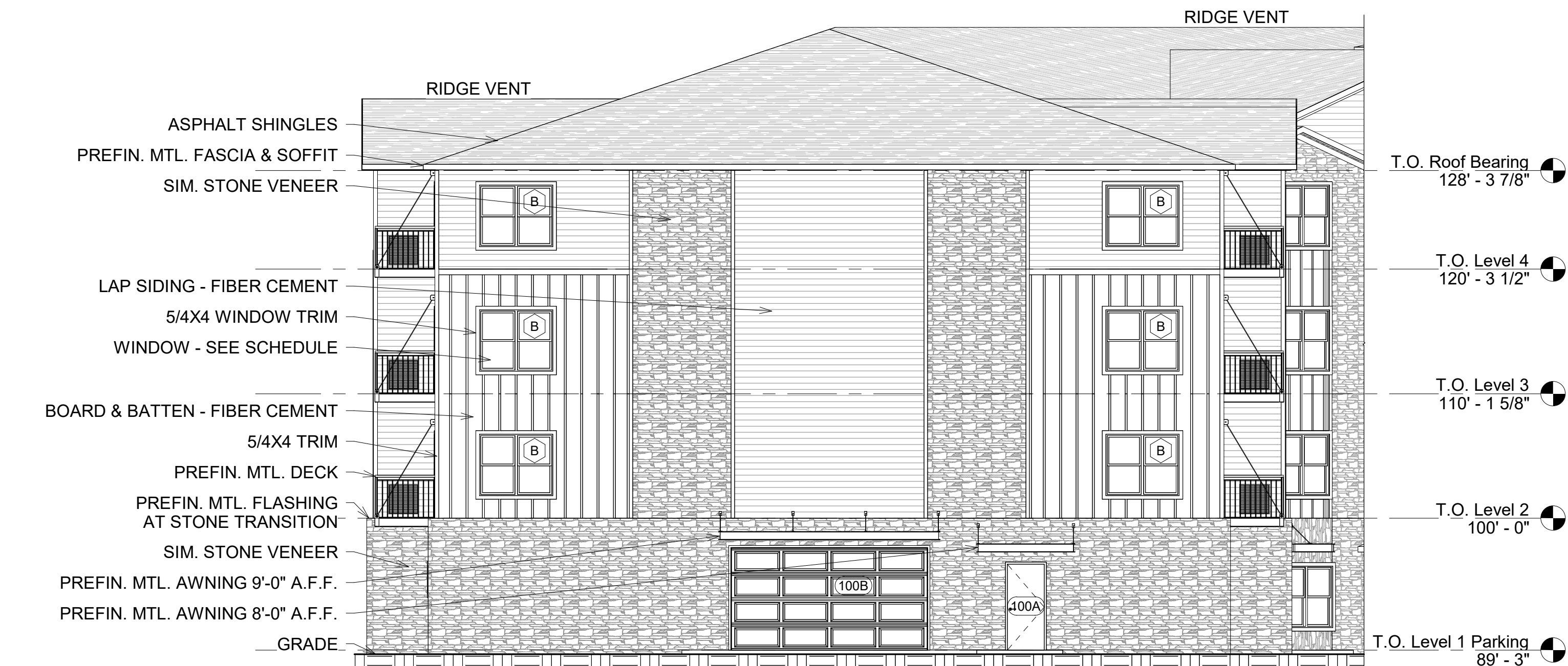
1 Enlarged Building Elevation - West 1 1/8" = 1'-0"
