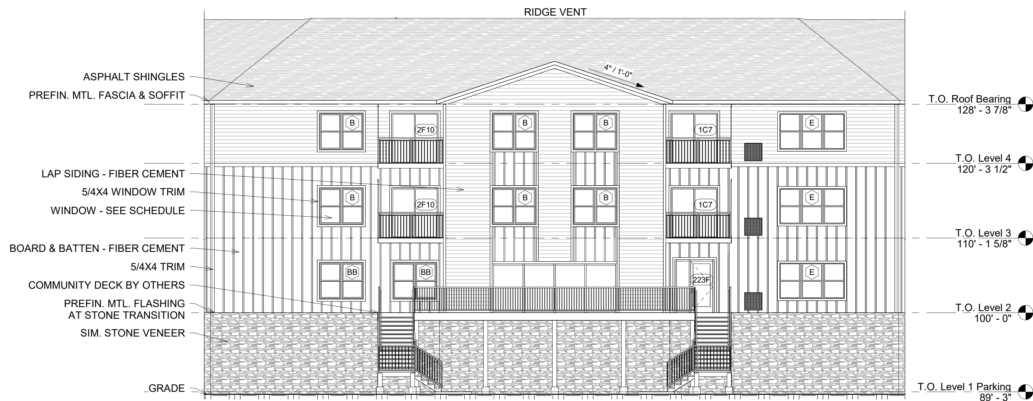
1 Enlarged Building Elevation - North West 1/8" = 1'-0"
