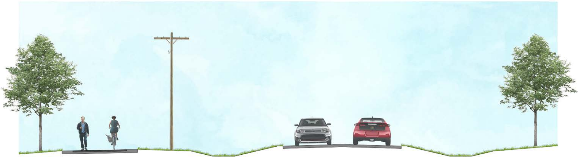
Illustrative roadway corridor showing 10' multiuse trail at left, utility corridor with appropriate setbacks, and 22' two-way roadway
