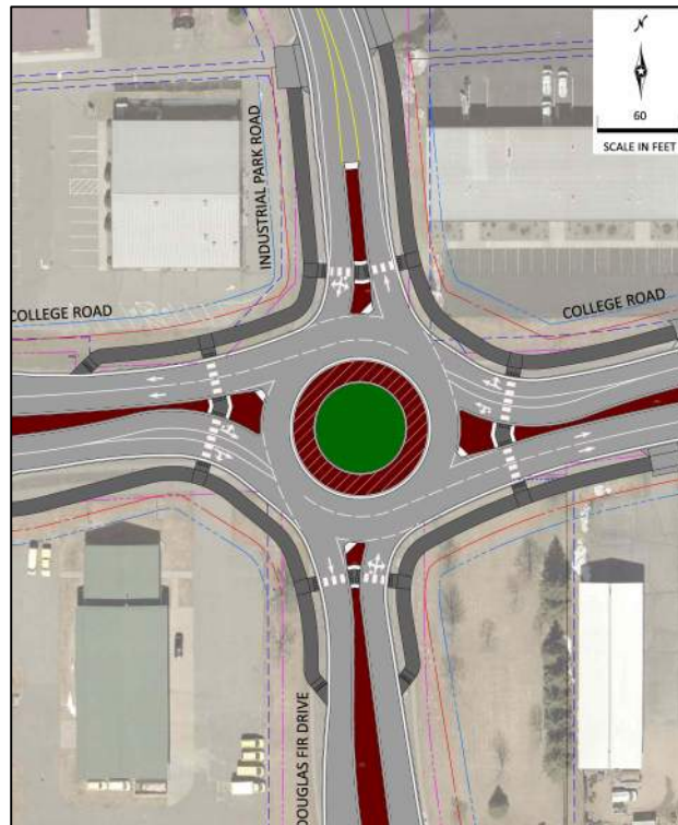
Figure 10 – Douglas Fir Drive Roundabout Preliminary Layout
