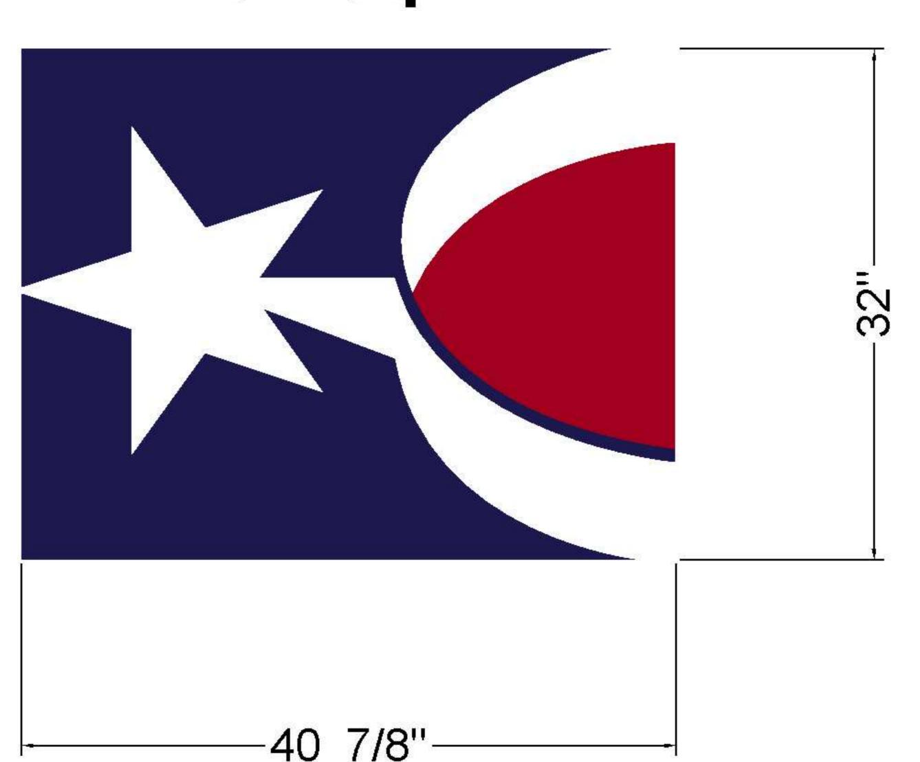
(1) Set of 13.5" tall, black, non-illuminated metal letters (1/4" thick) (1) 32" tall non-illuminated metal logo (1/4" thick) Mounted with studs, to stand off 1" from building surface.
