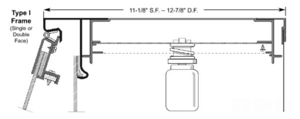
Inside sign cabinet, is a 120VAC standard base 300 lumens, 40-watt equivalent, (not to exceed) 3000K LED bulb controlled by timer.
