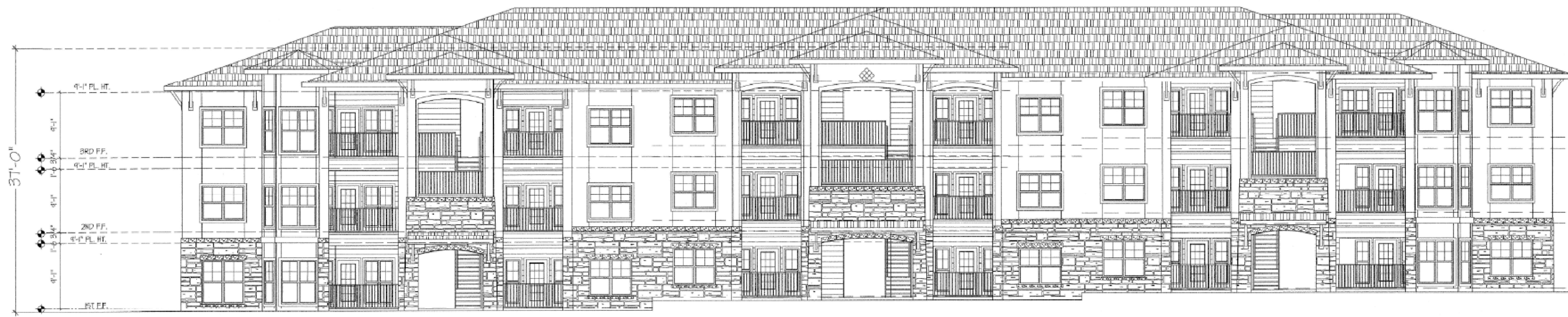
TYPICAL BUILDING FRONT ELEVATION NOTE: BUILDING HEIGHT IS MEASURED FROM AVERAGE SITE GRADE. 1" = 16'
