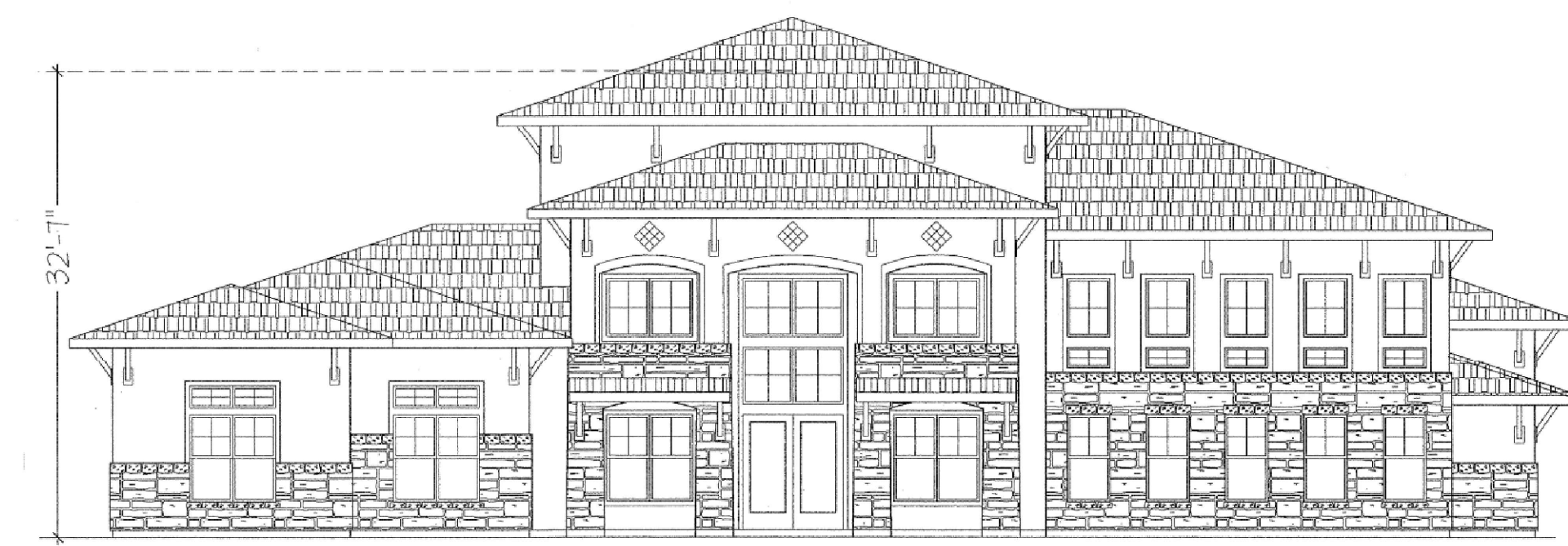
CLUBHOUSE FRONT ELEVATION NOTE: BUILDING HEIGHT IS MEASURED FROM AVERAGE SITE GRADE. 1" = 16'
