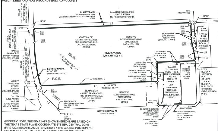
THE TEXAS STATE PLANE COORDINATE SYSTEM, CENTRAL ZONE (FIPS 4203) (NAD'83), AS DETERMINED BY THE GLOBAL POSITIONING SYSTEM (GPS). ALL DISTANCES SHOWN HEREON ARE ON THE SURFACE. THE COMBINED GRID TO SURFACE SCALE FACTOR FOR THE PROJECT IS 1.0000139976. THE UNIT OF LINEAR MEASUREMENT IS U.S. SURVEY FEET.
