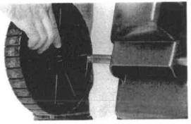
Quick Release Wheels make handling swaps and exchanges a simple task
