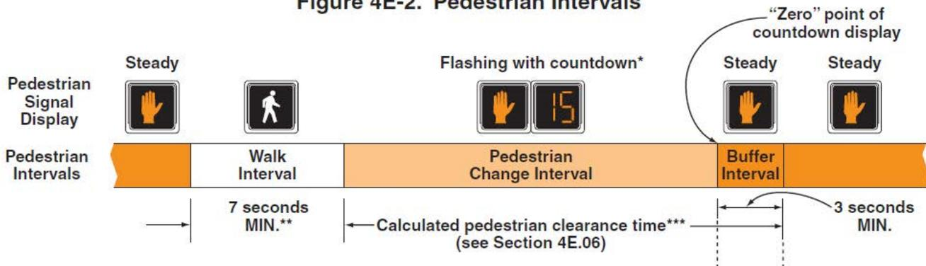
If pedestrian signals are installed at an intersection, they should include a countdown display to warn pedestrians how much time they have left to cross.
