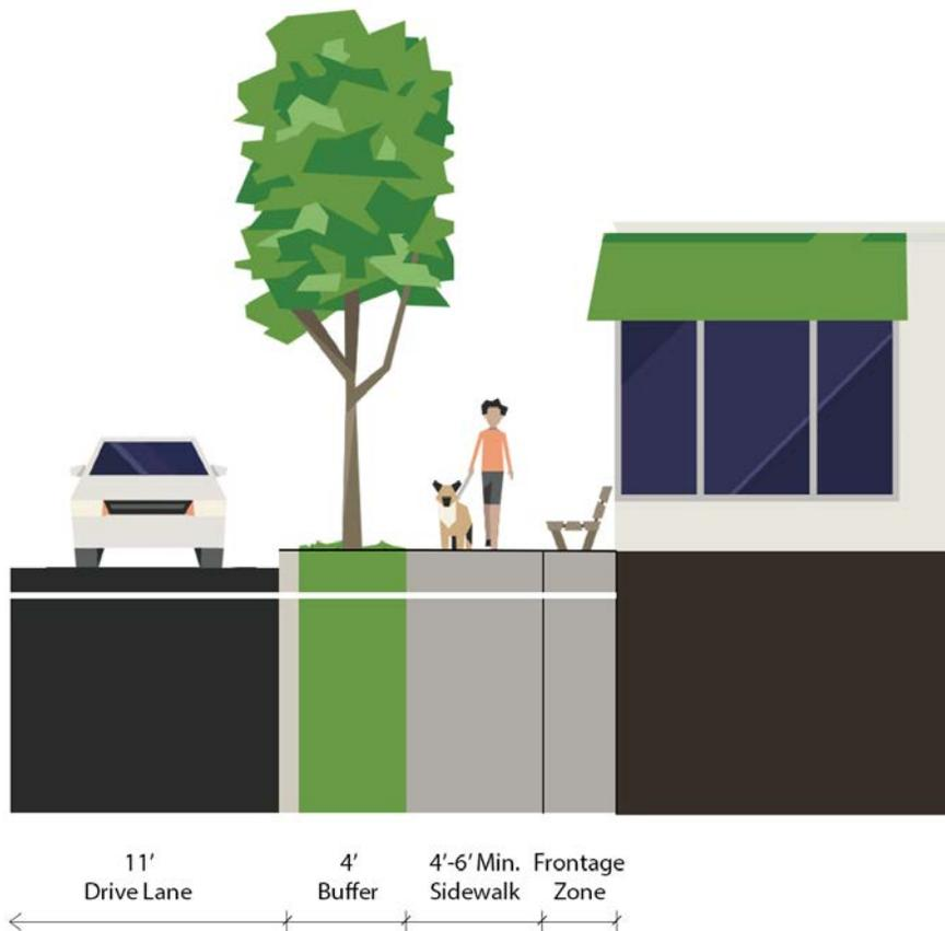
The pedestrian access route (sidewalk) should be at least four feet in width (preferably five to six feet) and kept clear of obstructions such as doors, table/benches, signs, and vegetation. The pedestrian access route is typically accompanied by a frontage zone adjacent to the building face, providing room for benches, cafe tables, lighting, and signage.
