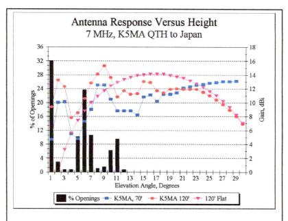
Fig 10—Elevation response on 7 MHz from K5MA location towards Japan on 7 MHz. The 120-foot high Yagi is definitely superior to the one only 70-feet high.
