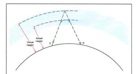
Fig 1—A simplified cross-sectional representation of ionospheric propagation. The simple triangle goes from the Transmitter T up to the virtual height and then back down to the Receiver R. Typically the F layer exists at a height of 150 miles above the Earth at mid-latitudes. The distance between T and R may range from a few miles to 2500 miles under normal propagation conditions.
