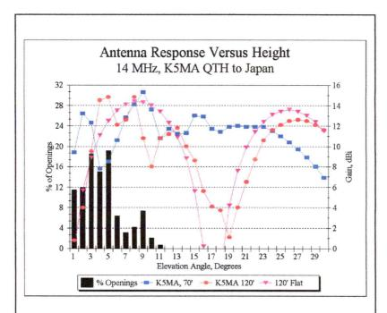
Fig 9—Computed elevation responses of 120- and 70-foot high Yagis, at the K5MA location on Cape Cod, in the direction of Japan and over flat ground, for comparison. The elevation response of the real-world antenna has been significantly modified by the local terrain.
