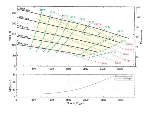
Pump Make Pioneer Pump Pump Model PP66S14 Operating Speed Variable Min. Speed 1200 rpm Max. Speed 1950 rpm Impeller Rated Dia. 14 inch Impelier Type **Enclosed** No. of Impelier Vanes 2 Solid Dia 3 inch Specific Speed 1832 US Units Suction Size 6 inch Discharge Size 6 inch
