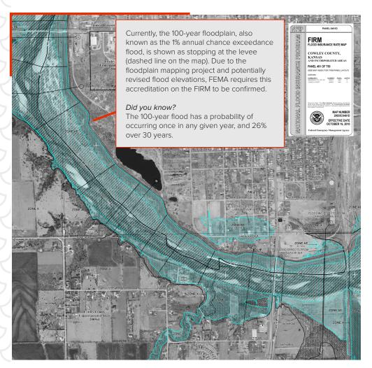
FEMA requires the freeboard for the top of the levee to be a minimum of three-feet higher than the 100-year floodplain. The certification process will include review of this criteria.
