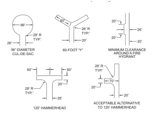
Show all turning radius are a minimum of 35 feet inside and 55 feet outside face of curb. (2018 IFC 503.2.4)
