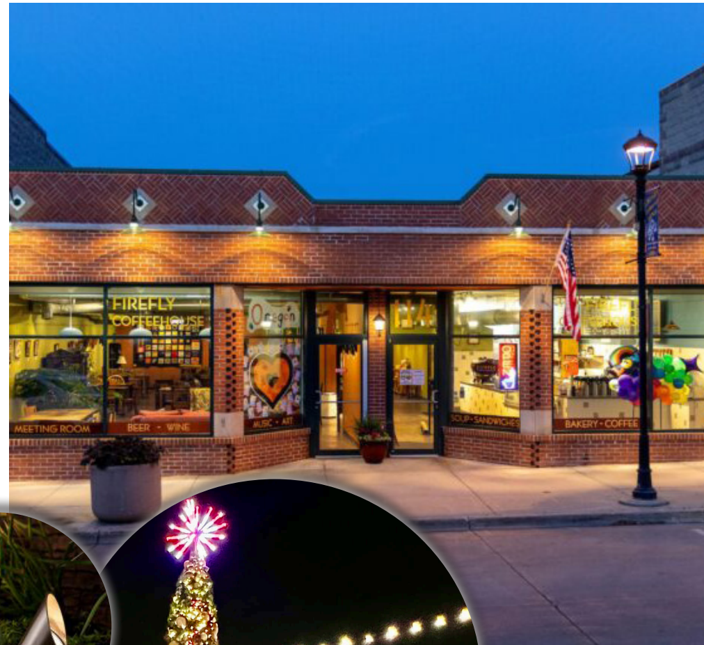
▲ Utilize downlighting mounted to building walls and structures to reduce light pollution and provide an aesthetic experience.
