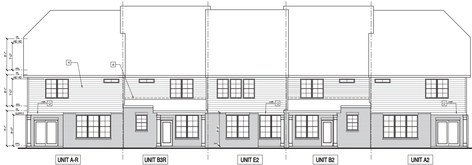
Rear Elevation 5-Plex 'B' SCALE: 3/16"=1'-0" AT 22"x34" LAYOUT
