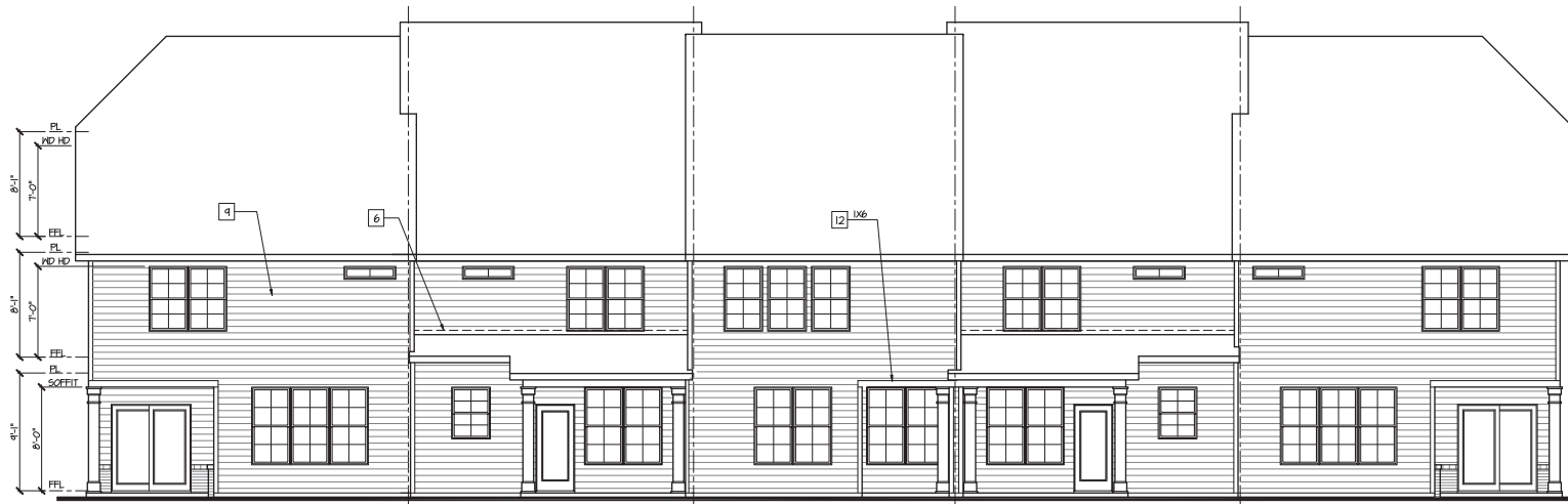
UNIT A-R UNIT B3R UNIT E2 UNIT B2 UNIT A2 Rear Elevation 5-Plex 'B'
