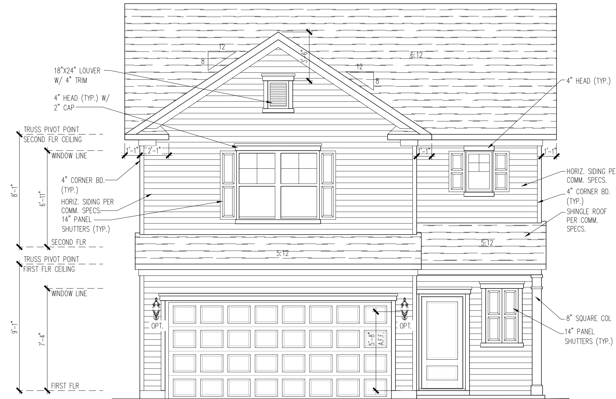
FRONT ELEVATION "LC1A" FRONT ENTRY GARAGE
