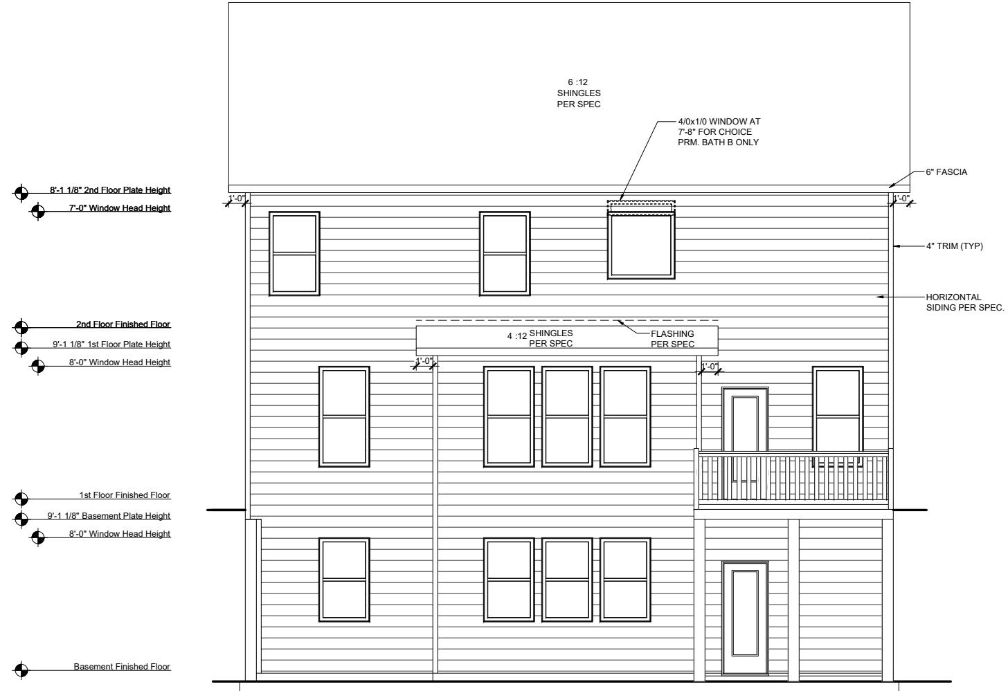
REAR ELEVATION AT BASEMENT SCALE: 1/8"=1'-0" (11"x17" SHEET SIZE) SCALE: 1/4"=1'-0" (24"x36" SHEET SIZE)
