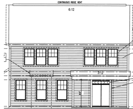
REAR ELEVATION 'B' SCALE: 1/8"=1'-0" OR 11/16"
