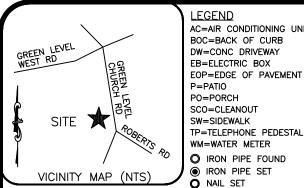
**LEGEND** AC=AIR CONDITIONING UNIT BOC=BACK OF CURB DW=CONC DRIVEWAY EB=ELECTRIC BOX EOP=EDGE OF PAVEMENT P=PATIO PO=PORCH SCO=CLEANOUT
