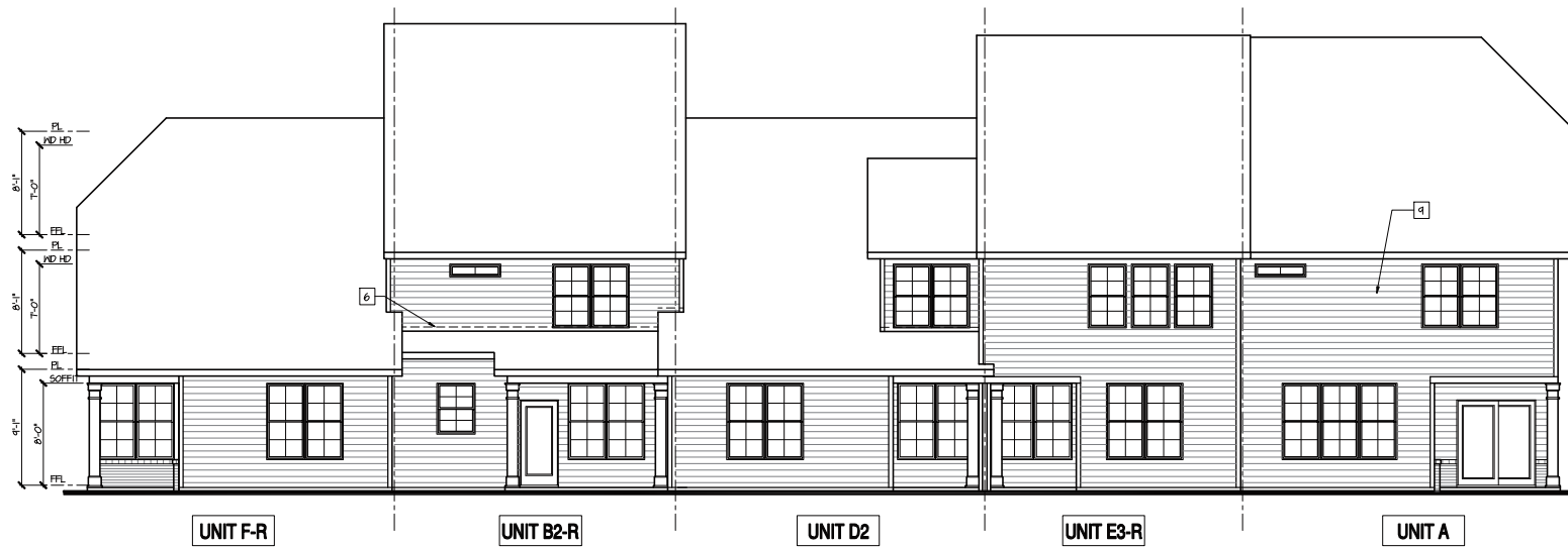
Rear Elevation 5-Plex 'A'
