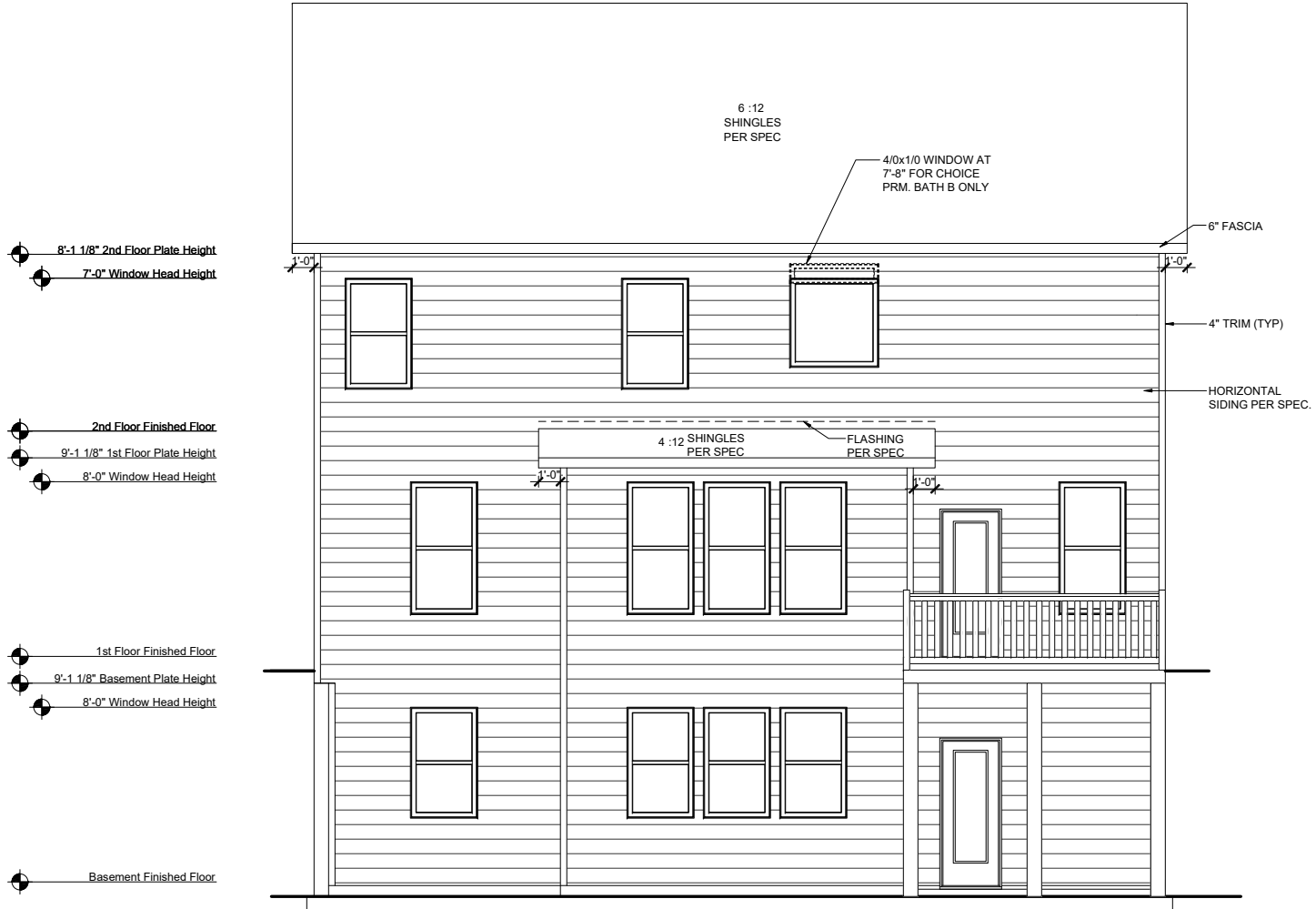
REAR ELEVATION AT BASEMENT SCALE: 1/8"=1'-0" (11"x17" SHEET SIZE) SCALE: 1/4"=1'-0" (24"x36" SHEET SIZE)
