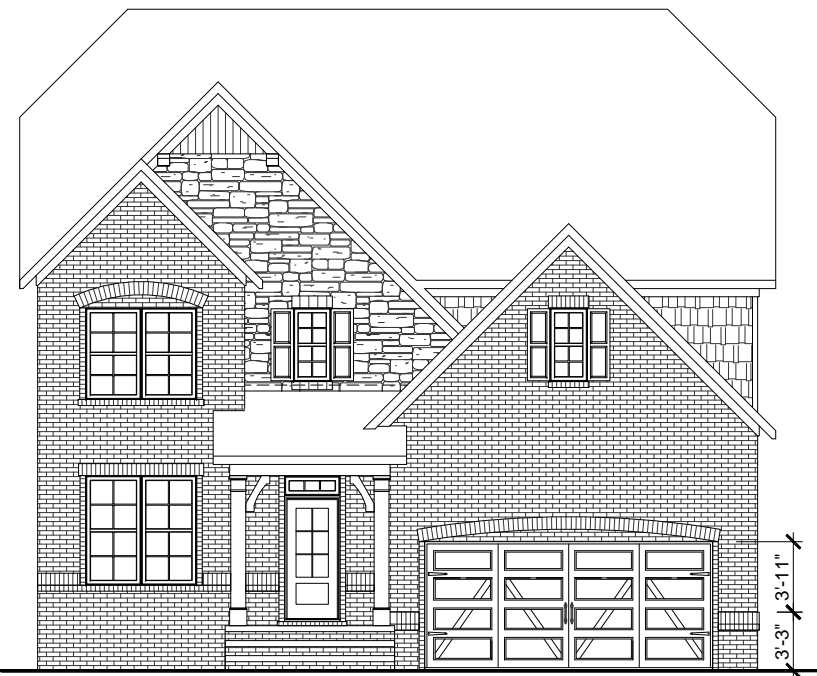
FRONT ELEVATION - FCL on CRAWLSPACE SCALE: 3/32"=1'-0" (11"x17" SHEET SIZE) SCALE: 3/16"=1'-0" (24"x36" SHEET SIZE)
