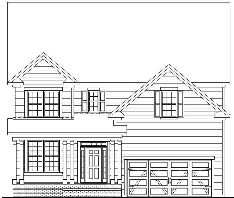
FRONT ELEVATION - TRA on CRAWLSPACE SCALE: 3/32"=1'-0" (11"x17" SHEET SIZE) SCALE: 3/16"=1'-0" (24"x36" SHEET SIZE)
