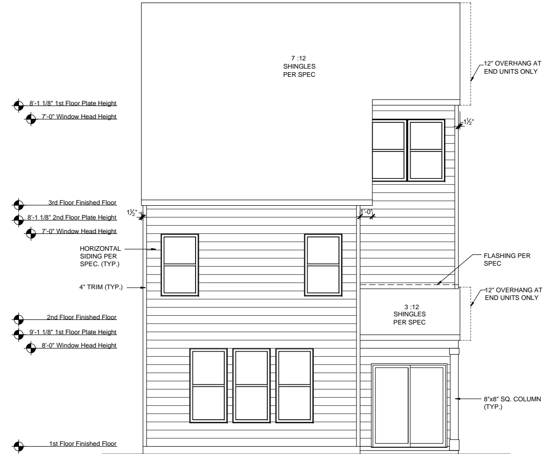
REAR ELEVATION W/OPT. COVERED PATIO SCALE: 1/8"=1'-0" (11"x17" SHEET SIZE) SCALE: 1/4"=1'-0" (24"x36" SHEET SIZE)
