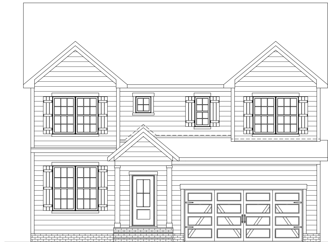
FRONT ELEVATION TRL ON CRAWL SPACE SCALE: 1/8"=1'-0" (11"x17" SHEET SIZE) SCALE: 1/4"=1'-0" (24"x36" SHEET SIZE)
