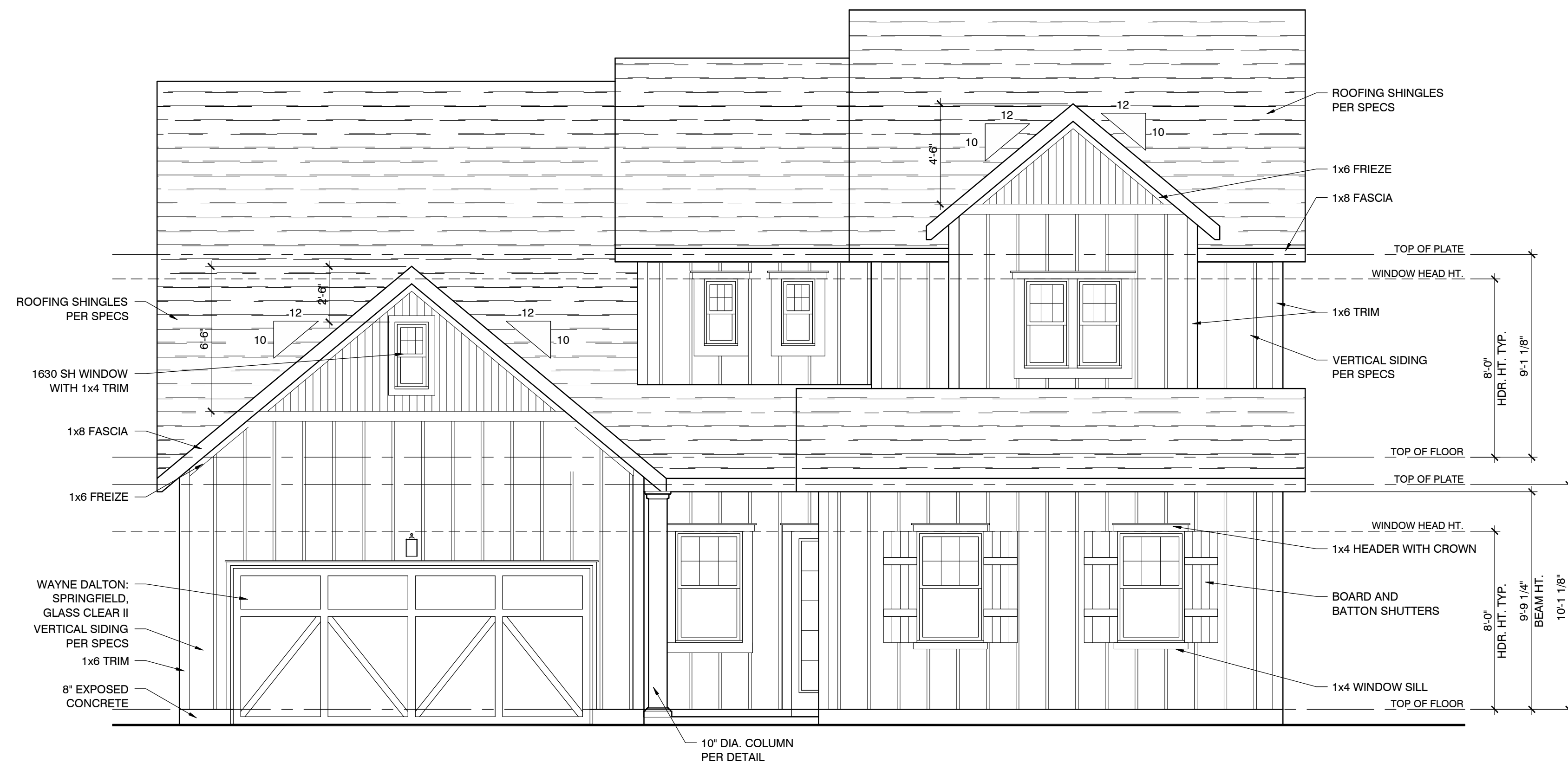
FRONT ELEVATION - PLANK COTTAGE SCALE: 1/4"=1'-0"
