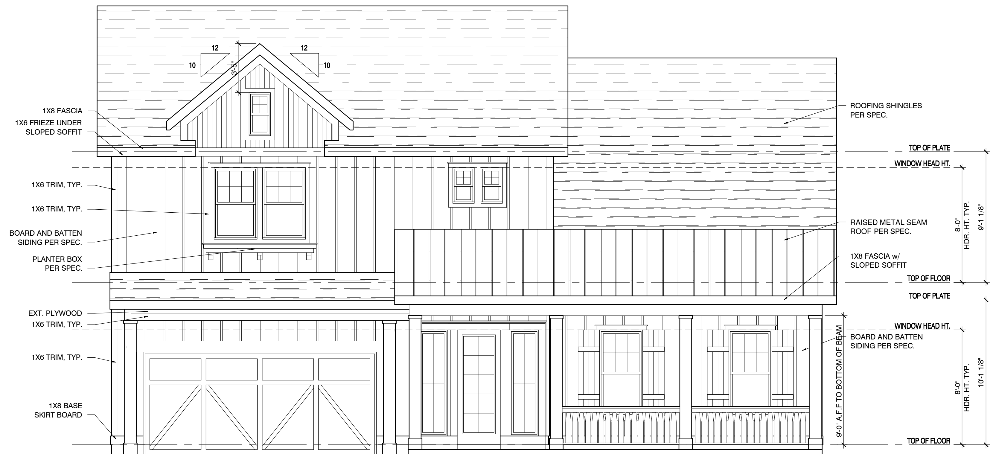
FRONT ELEVATION - PLANK COTTAGE SCALE: 1/4"=1'-0"
