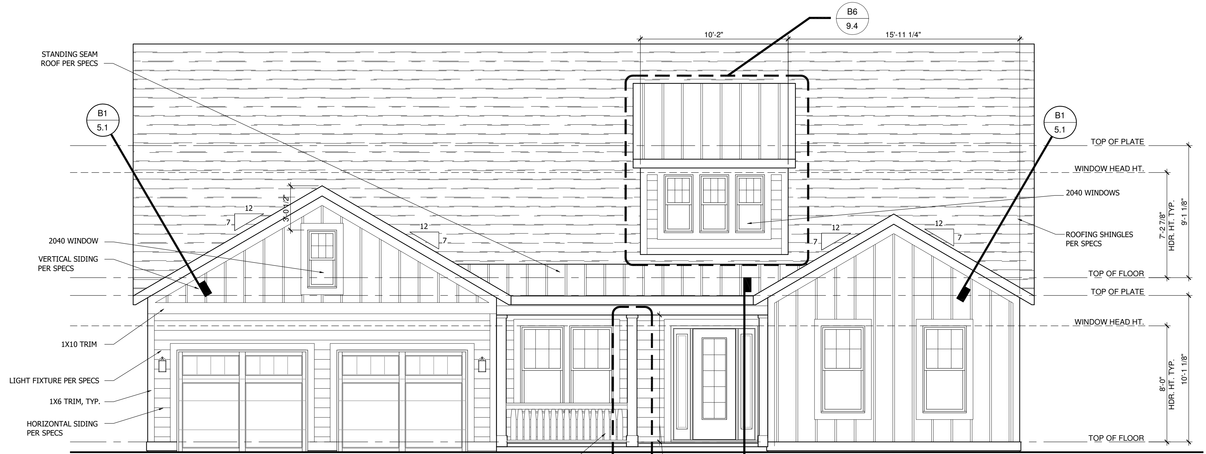
FRONT ELEVATION - PLANK COTTAGE SCALE: 1/4"=1'-0"
