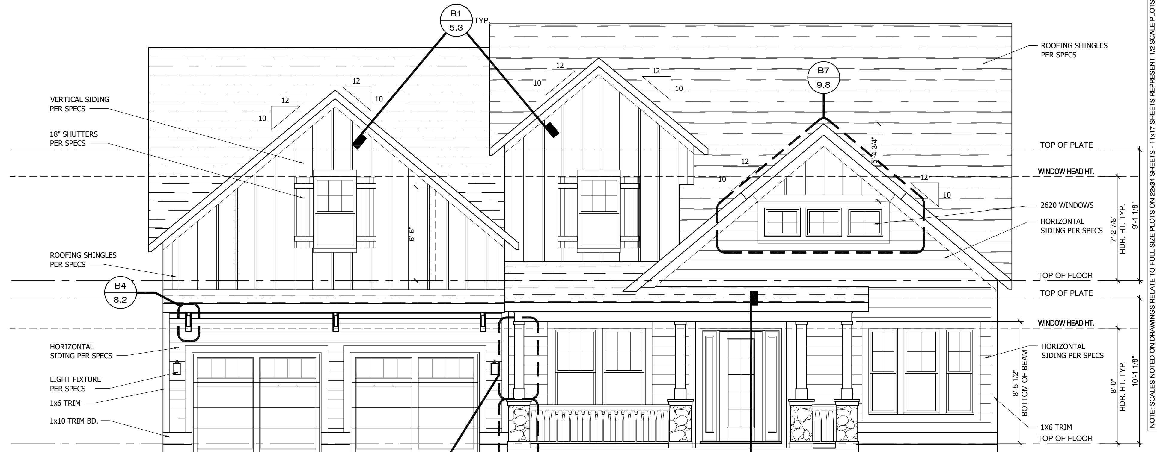
FRONT ELEVATION - PLANK COTTAGE SCALE: 1/4"=1'-0"
