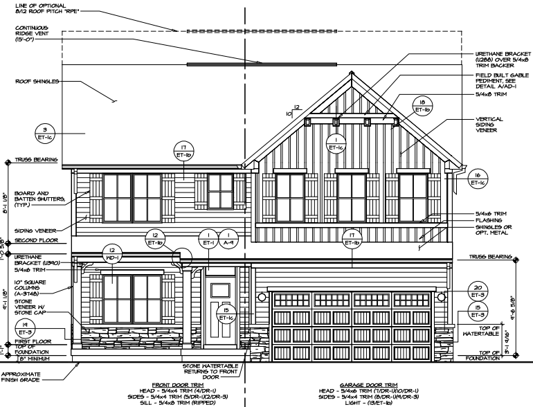
4 FRONT ELEVATION "K" SCALE: 1/4" = 1'-0" TWO CAR FRONT ENTRY GARAGE "SC2" PORCH EXTENSION "EP3"
