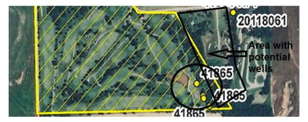
The map above shows the 3 wells, their geographical center and a 600 foot diameter circle around the geo-center. A battery of wells can be up to 4 wells all within a 600 foot diameter circle.
