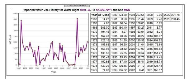
The DWR data above shows the water usage for the water right that covers all 5 wells. It shows the City has 400 AF of water rights. Historically the City uses 200 AF or less per year.
