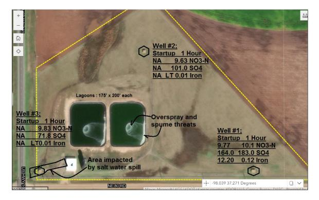
The lab data for these wells indicate Nitrates hover around the 10 mg/L value. The sulfates increase with pumping in Well #1 and are significantly higher than Wells #2 and #3. Again, this increase in Sulfates may impact plant efficiencies.
