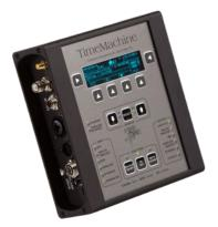
GPS sync TimeMachine provides 0.01 second accuracy for soundtrack broadcast to the Radio Station and local sound systems and each event location
